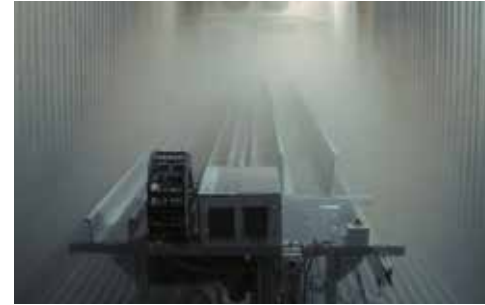
Cold test at -40°C for chainflex® cables and e-chains®.
