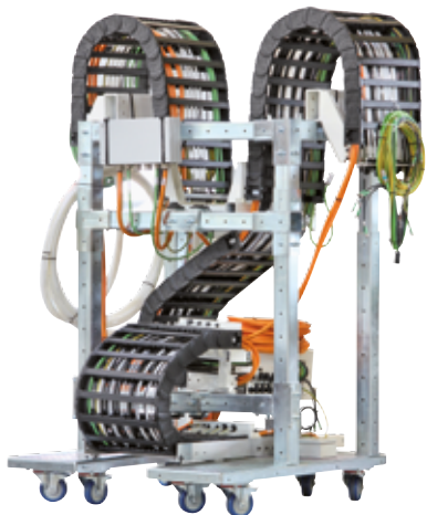
Harnessed igus® readychain® system for textile machines.
